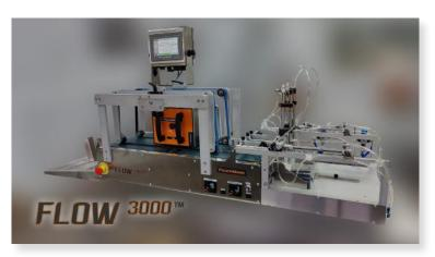
the FLOW 3000 is as close as you can get to a perfect solution. Print everything from nutrition panels, compliance data, production codes, logos, text and virtually any type of barcode directly onto pre-formed pouches, eliminating the need for pre-printed, hand- or machine-applied labels.
