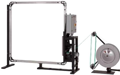
The MOD-710 side seal plastic strapping machine combines quick-change technology with high speed reliable operation to maximize productivity. Simple to operate and easy to maintain, the MOD-710 features a modular head with separate tensioning and sealing modules that are easy to access and can be changed out quickly for routine maintenance. The MOD-710 is available in 69 standard chute sizes and uses Contrax polypropylene or Tenax polyester strapping. Made in the U.S.A.
