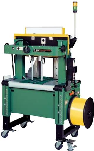
Loaded with productivity enhancing features, the LBX-Magazine™ minimizes downtime, simplifies maintenance and virtually eliminates make-ready time between magazine runs. The hinged bundle handling device can be pivoted up to 90°, providing complete access to the tabletop and strapping head for maintenance. Made in the U.S.A.
