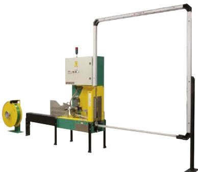
The MH-VRB side seal plastic strapping machine applies consistent, high strap tension to palletized loads in a wide range of sizes. The MH-VRB can be used with 9 mm or 10.5 mm polypropylene or polyester strapping to accommodate a variety of load types, including cartons, palletized products, appliances, bulk bins, bales and bundled items.
