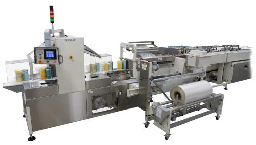
The 914OVS servo orbital vertical sealer is the machinery solution of choice for end-of-filling-line shrink packaging. Now products such as bottles, jars or cans are able to be wrapped while in the vertical position.
