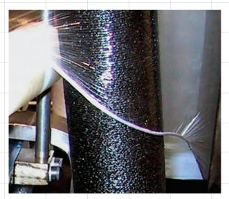
Pallet Grip rolls 4" to 6" of the film web into a tight, high strength, durable film cable.
