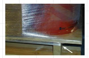
The rolled up film cable is driven down on the pallet to about an inch and a half below the topboards, where it can't be damaged by fork truck entry.
