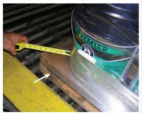
Product is securely wrapped and tightly "locked" to the pallet with the film cable produced by Pallet Grip. The high strength film cable prevents the load from sliding off the pallet.
