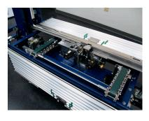
The CB4000 in line corrugated bundler incorporates the latest servo motor technology that provides the ultimate in reliability. This technology also provides high speed production rates, 40% less moving parts and minimal maintenance requirements. The CB4000 includes
