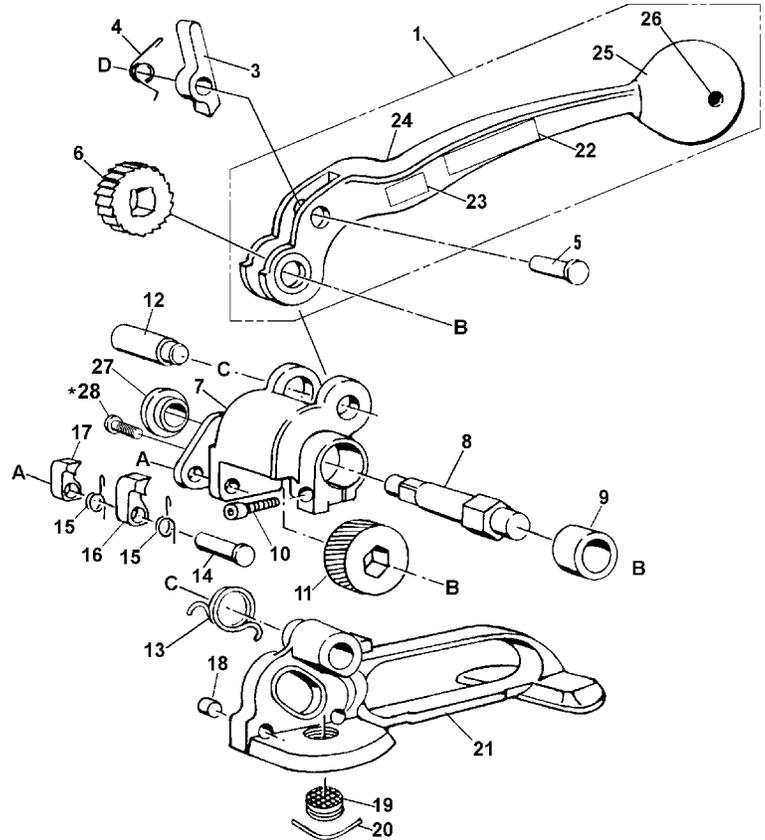
When ordering parts, please show tool model, part number, and description. All recommended spare parts are underlined and should be stocked.
