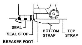
Pull back on the TOP STRAP to eliminate additional slack around the package. You will have to push on the cylinder cover to make certain that the jaw tips are in position over the seal.
