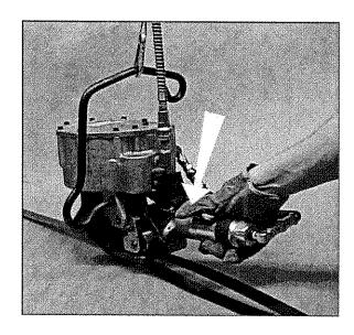
If strap alignment is unsatisfactory and it becomes necessary to shut off the tool during the tensioning portion of the cycle, push down on the stop lever.
