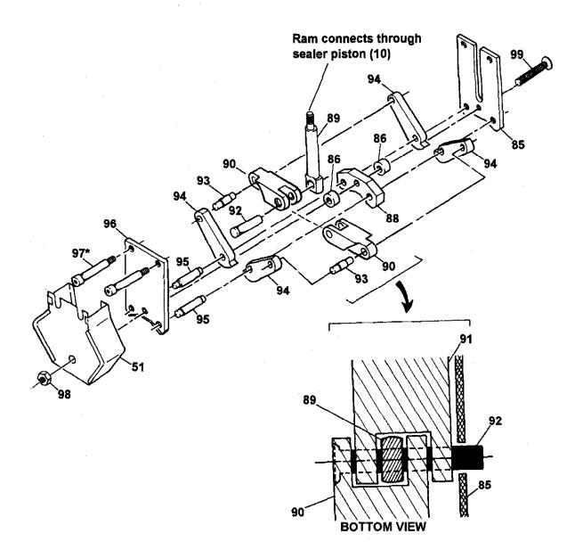
\* Apply one drop of Loctite #242 sealant to cleaned parts. Allow 12 hours to set, if possible. Do not apply to small screws or close moving parts as the fluid spreads easily.
