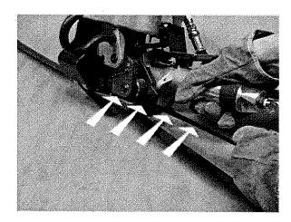
Push the tool forward until the seal-stop contacts the end of the seal.
