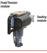
The MH-VR and VRB machines utilize the revolutionary MHC modular strapping heads. Designed for reliable, low maintenance operation, the MHC strapping head features separate lightweight sealing and tensioning modules that are easy to access and remove for maintenance. When switching to a spare module, the MH-VR and MH-VRB can be up and running in minutes.
