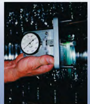
A tensometer is used to check the strap tension on can and bottle loads
